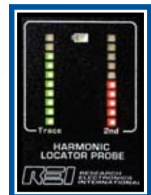
Close-up of HLP display showing wire-trace level (green) and 2nd harmonic response level (red) indicating electronics.
