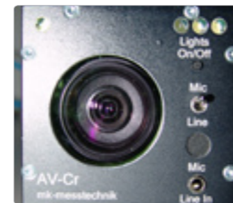
Front of camera module including microphone and LED lighting
