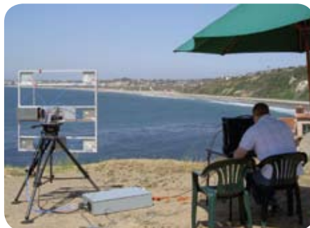
Reflectometer array provided precision velocity measurement for munitions trials
